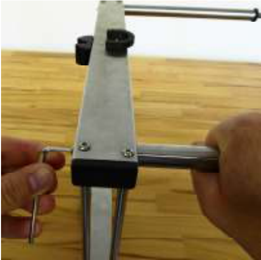
Fig. 2.8. Legs assembled on frame
