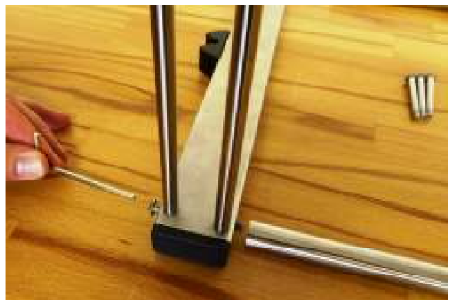
Fig. 2.5. Fixing leg into frame with allen key 3mm
