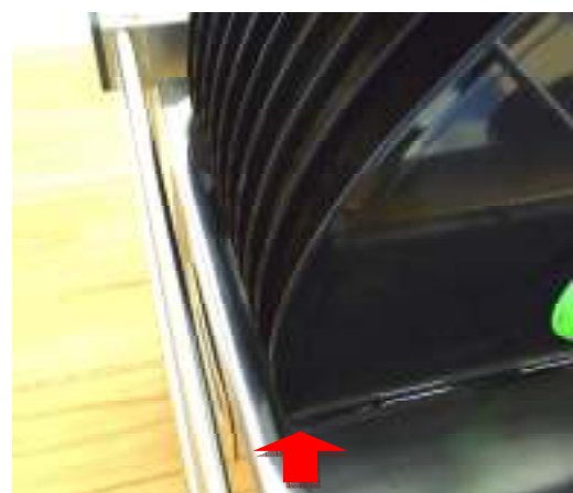
Fig. 9.5. Gap between edge of bath and LPs
