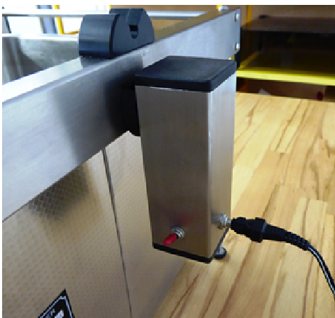
Fig. 5.0. Motor, switch, plug in DC supply
