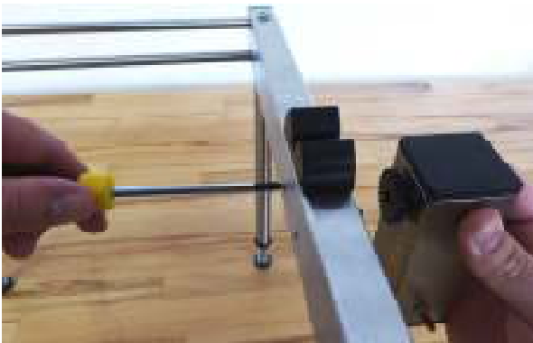
Fig. 3.0. Frame with motor ready for mounting
